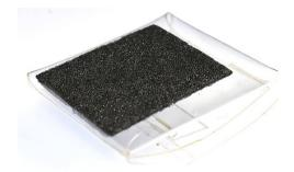
2. Slowly remove the foam sample from the box to minimize the generation of static charges as the foam slides out of the box.
