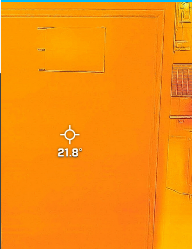
The top-right image is a front-on visual representation to show how the graphene is placed on the back of our prototype dry wall heater. The thermal scans - taken about five minutes apart - show a temperature rise > 20°C.
