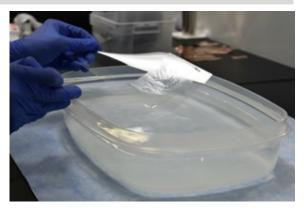
2. Please note that handling graphene on a support polymer is a difficult process, and various issues including insufficient/thin PMMA, insufficient drying time, wrinkles in the transfer film, substrate adhesion issues may occur.
