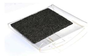
2. Use a sterile tweezer and hold carefully from one end to avoid damaging the 3D graphene foam.
